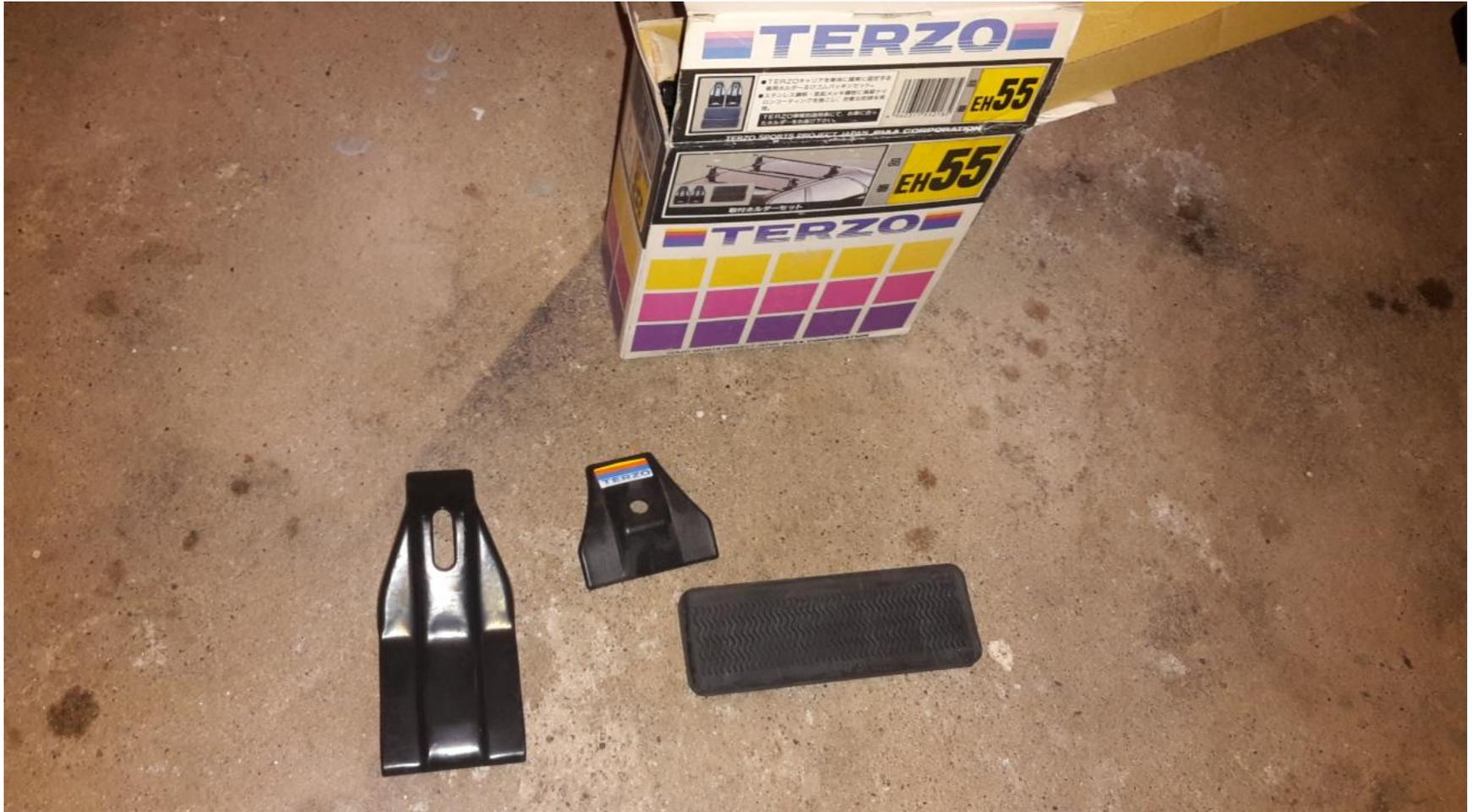
This is needed for mounting the system on cars with frameless windows
